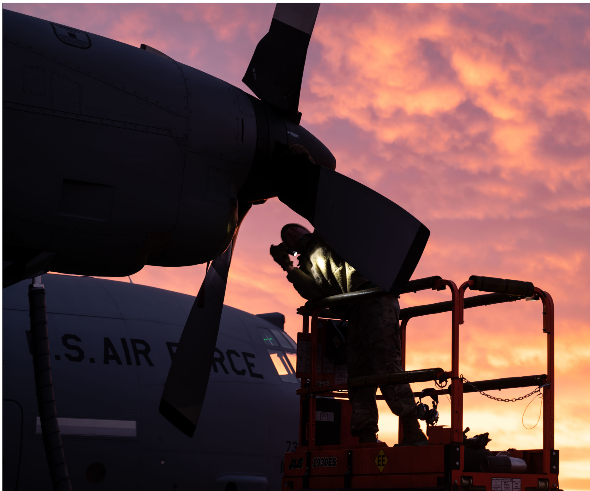
Air Force Master Sgt. Chad Wink, an airlift and special mission aircraft maintenance craftsman assigned to the 103rd Maintenance Group, applies heat to a C-130H aircraft propeller, December 13, 2021, East Granby, Connecticut. At sunrise, members of the 103rd Maintenance Group prepared the aircraft for flight. (U.S. Air National Guard photo by Master Sgt. Tamara R. Dabney)
