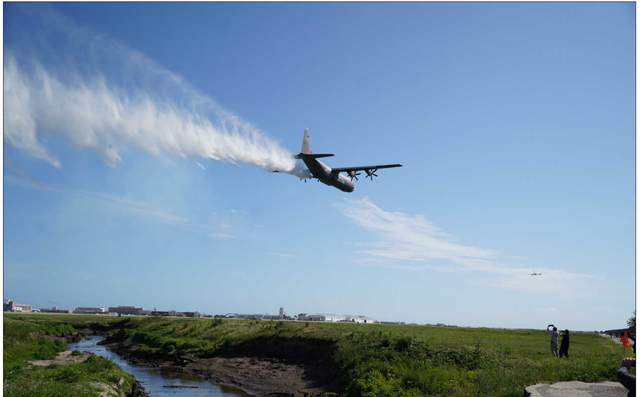
A California Air National Guard C-130J Super Hercules aircraft, assigned to the 146th Airlift Wing, equipped with the Modular Airborne Fire Fighting System (MAFFS) performs a water drop during MAFFS training at Channel Islands Air National Guard Station, Port Hueneme, California, April 24, 2024. Air National Guard aircrew from the California Air National Guard's, 146th Airlift Wing and the U.S. Air Force Reserve's 302nd Airlift Wing, train together to accomplish their aerial firefighting certification alongside the U.S. Forest Service and other wildfire prevention agencies. The recertification training includes classroom sessions, flying and ground operations for Air Force aircrews, civilian lead plane pilots, and support personnel from the Forest Service, Bureau of Land Management, and other federal and state agencies. (U.S. Air National Guard Photo by Tech. Sgt. Michelle Ulber)
